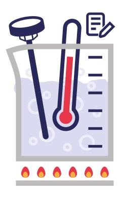
Reread the temperature of the boiling water using the calibrated thermometer at least two to three times and record results on a logbook. Wash the thermometer with room temperature water in between readings.
