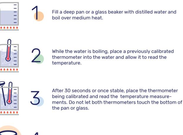
If the temperature readings are not the same, ideally 212°F (100°C), adjust the nut until the reading is correct\*.
